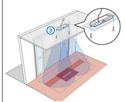
**Step 3**: Mount the plate with camera on the wall with 2x screws and wall plugs.
