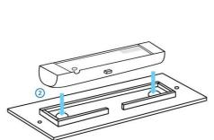
How to Install Flush Mounting Plate
