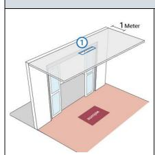
Step 1: Determine the mounting location (ideal height: 2.8m – 3.5m), cut the hole of camera space for installing the mounting plate (264mm x 70 mm)
