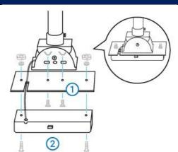
**Step 1**: Attach the mounting plate to the drop pole using the internal screws, then attach the counter to the mounting plate using the external screws.
