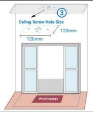
**Step 2**: Determine the mounting location and drill **(5)** holes for installing the drop pole. The holes should be drilled within **(120mm x 120mm)**
