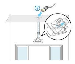
**Step 4**: Connect the Cat5 cable through the tubes of the drop pole.
